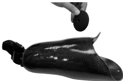
Manufacture the socket using the appropriate Blatchford single bolt former. Cut a 27 mm diameter hole in distal end of socket. Place socket plate inside socket. Assemble alignment parts supplied. Minimum socket thickness 6 mm.
