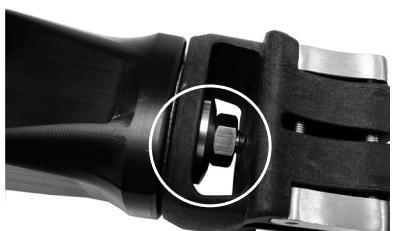
Apply Loctite 243 to bolt threads. Assemble the distal top housing using the nut and washer as shown and torque tighten to 35 Nm after alignment.
