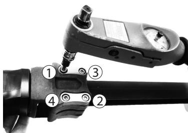
Tighten clamp screws evenly, applying a torque of 5 Nm at least twice to each screw. Example order of tightening shown to evenly spread load.
